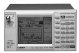
**Model 953** offers both spectrum analyzer functions and multiple/single bargraph level readings for TV, CATV, FM, wireless mic and many other RF services covering the range of 5 to 1030 MHz. Totally portable and easily programmed, it combines the time saving power of auto search and ranging with lookup tables for broadcast and cable frequency assignments used in the USA and throughout the world.
