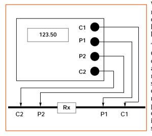
When measuring resistance below 100 ohms it is advisable to use a four wire measurement technique (fig. 1), this is often referred to as a Kelvin or Thomson configuration. By using this type of measurement configuration the connecting lead resistance is not included in the measurement, and the need for lead balancing and nulling is eliminated.
