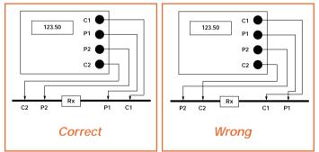
Most common cause of errors when making low resistance measurement are due to poor or inappropriate connection of the Rx. Connections should be clean, mechanically firm and free from oxides which can cause an insulating effect.
