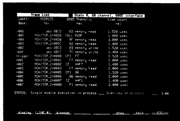
Figure 7. A listing of the state flow may be viewed in the mnemonics of the microprocessor code. Time and state counts are valuable analysis aids.
