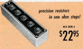
This precision Decade Resistance kit provides any resistance value from 1 ohm to 99,999 ohms . . . all at ½ of 1% accuracy. Twenty ½% precision resistors are arranged so that 5 rotary switches will select any value in one ohm steps. Switches are labeled "Units," "Tens," "Hundreds," "Thousands" and "Ten Thousands". Ideal for laboratory use in a multitude of experimental applications. 3 lbs.
