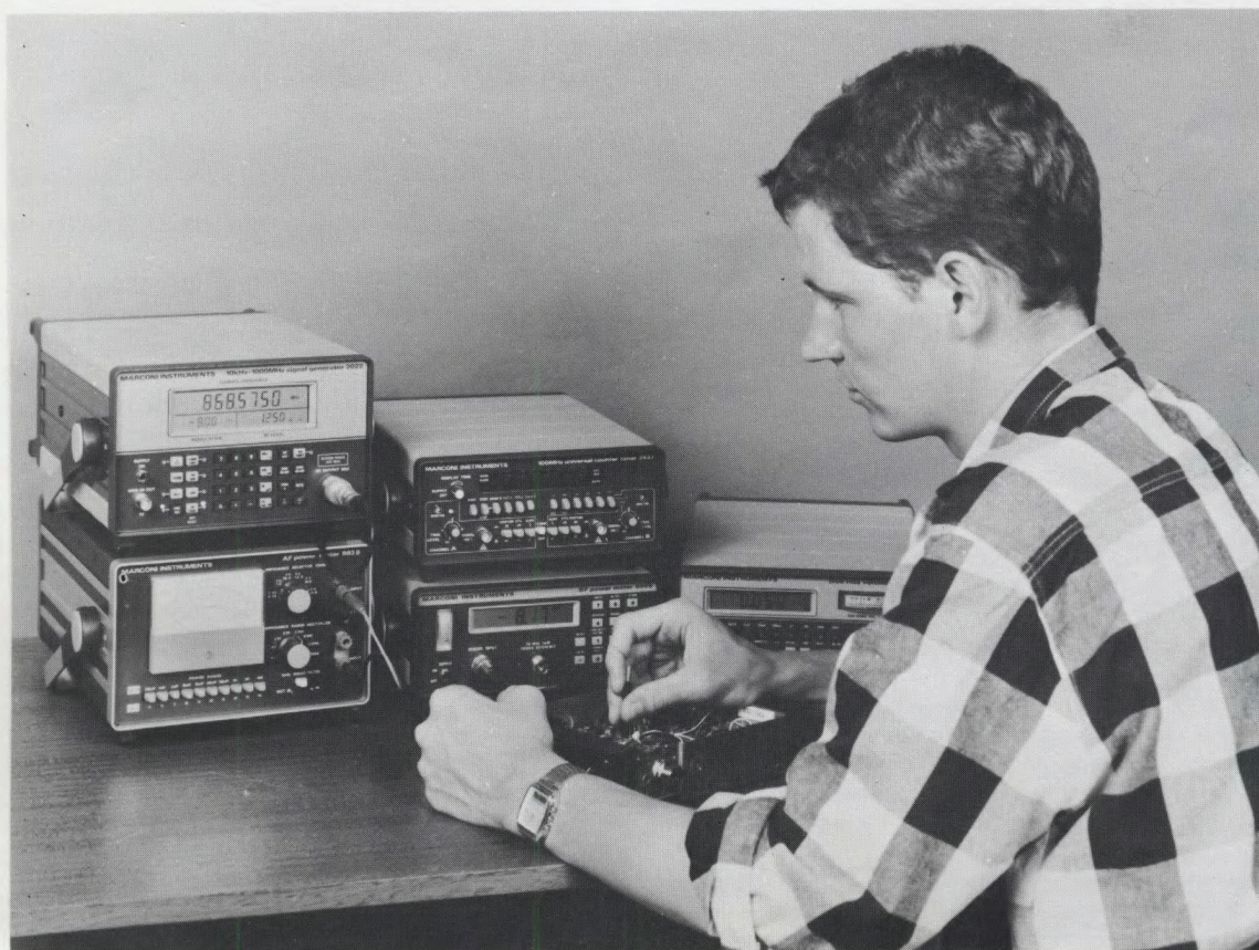
AM/FM Signal Generator 2022 is ideal for a variety of applications in receiver testing.
