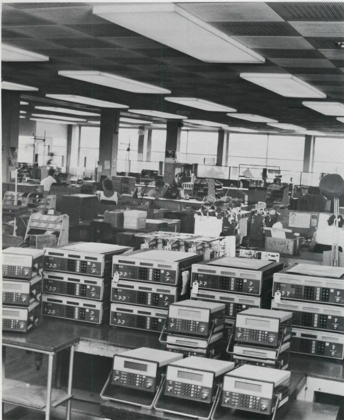
Simple calibration facilities and fast diagnostic functions enable rapid testing of Marconi Instruments' signal generators, here seen prior to final factory test. The same features are a significant factor in their low cost-of-ownership.
