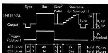
Waveform for general assessment (monochrome) with internal trigger
