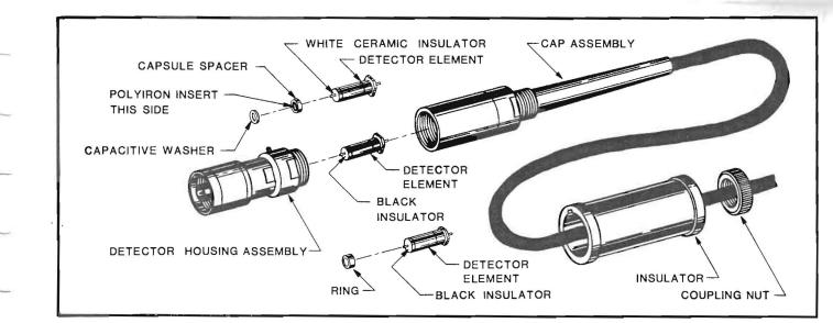
Figure 1. Element Replacement for Detectors Used With the 1038-H/V and 1034A Units
