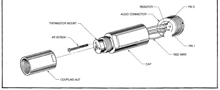
Figure 4. Resistor Replacement for Detectors Used With the Model 1045 Unit
