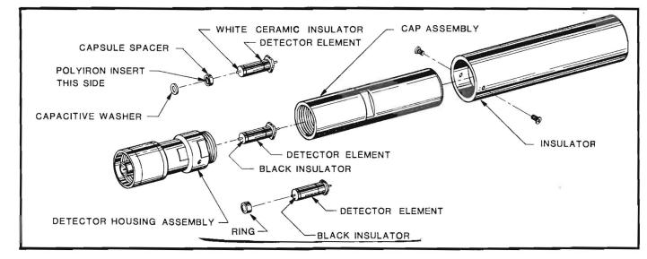
Figure 3. Element Replacement for Detectors Used With the Model 1045 Unit
