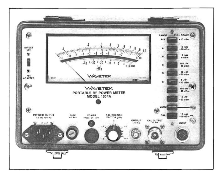
Figure 3-1. Model 1034A Front Panel
