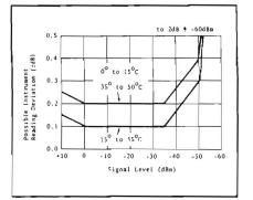
Figure 6 Model 1045 Detector Measurement Accuracy from 1MHz to 26.5GHz
