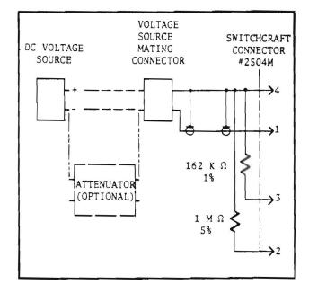
Figure 5-2. Fixture for Applying DC Voltage to the Model 1034A
