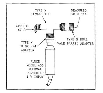
Figure 5-1. Modified Thermal Converter for Checking the Calibrator Output
