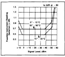
Figure 5 Model 1038-N10, NS20, and H/V Systems Waveguide Detector Accuracy from 28.5GHz to 40GHz
