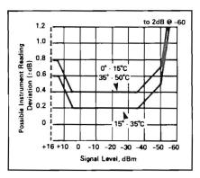
Figure 4 Model 1038-N10 and NS20 System Coaxial Detector Accuracy from 30MHz to 26.5GHz. (An additional 0.2dB is added to the deviation reading for operation from 1 to 30MHz)
