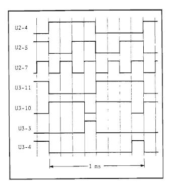
Figure 6-1. Chopper Circuit Timing Diagram
