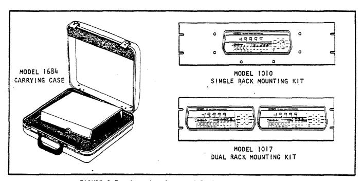
FIGURE 2-7. Carrying Case and Rack Mounting Kits.
