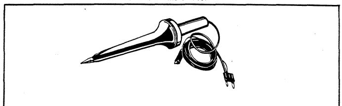
FIGURE 2-4. Model 1600 High Voltage Probe.
