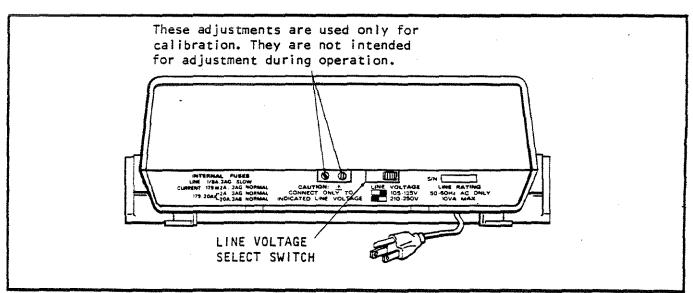
FIGURE 2-1. Rear View Showing Line Switch.
