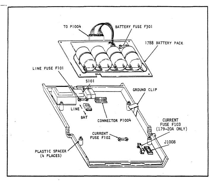
FIGURE 2-2. Battery Pack Installation
