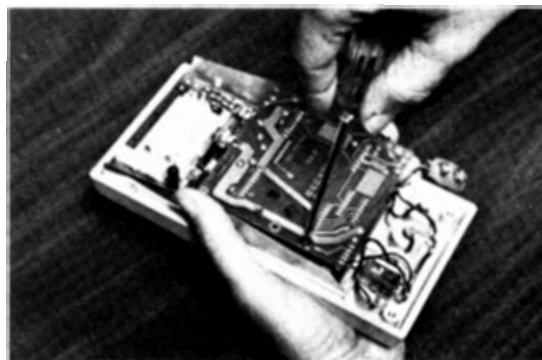
Figure 3-3. Disassembly and Replacement Procedure — Liquid Crystal Display and Multiprocessor Chip (continued)
