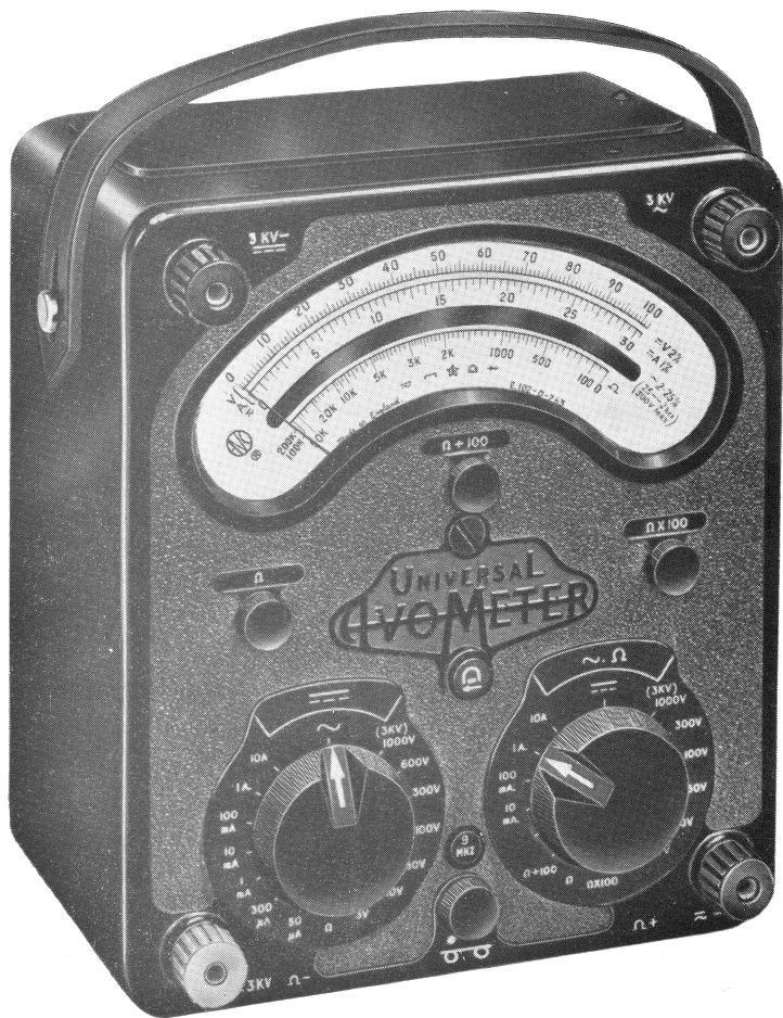
The Model 9 Avometer Mk. II
