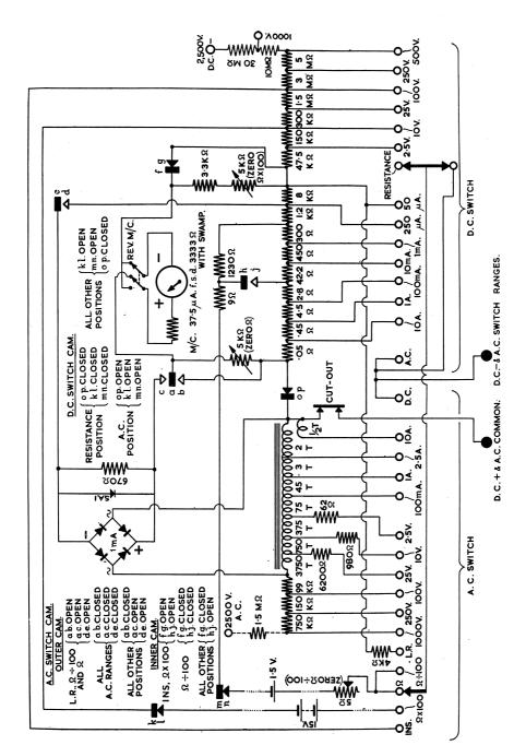
CIRCUIT DIAGRAM OF THE MODEL 8 AVOMETER MK. II
