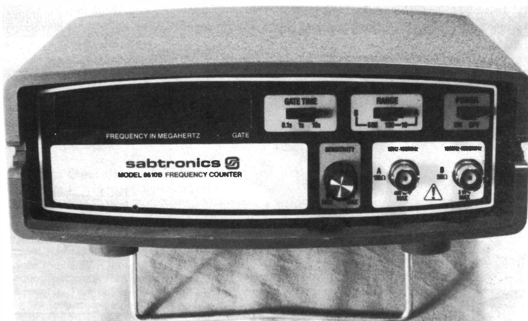
Fig. 1. The completed counter showing the clean, functional layout of the controls. The tiny hole just discernable beneath the letter E in 'Model' was drilled to gain access to the trimmer for adjusting the crystal oscillator frequency to exactly 10 MHz.
