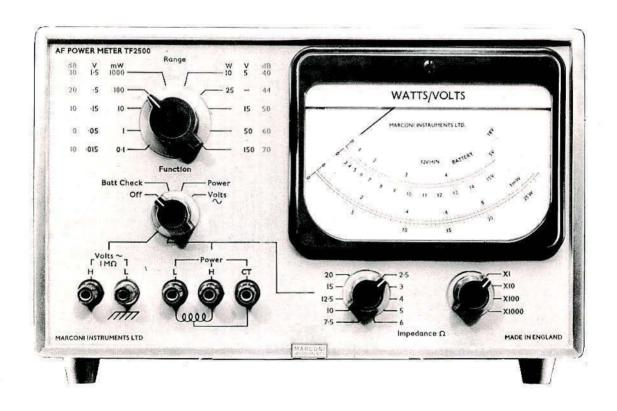
The TF 2500 is not only a wide range a.f. absorption power meter but also an accurate electronic voltmeter suitable for use up to 1 MHz. Furthermore, the voltmeter section can be used with external loading for direct measurement of power over the whole of its frequency range. In addition to the normal audio frequency power applications, therefore, the instrument can be used as a directly calibrated level monitor for a wide variety of transmission systems, including f.d.m. baseband networks.
