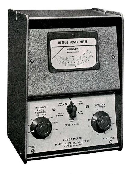
Power is measured by a temperature-compensated constant-resistance multi-range rectifier voltmeter, the required input impedance being obtained by the use of a tapped transformer and by a switched resistance-changing pad. Provision is made for measuring either balanced or un-balanced inputs.
