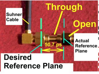
This is the hardware setup for the OPEN calibrating process:
