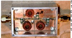
Since the current calibration is from 50kHz to 1500MHz this is a good object to measure. The picture shows the test piece. It is a printed circuit board with SMA connectors attached using right angle copper sheets. The inner conductors of the SMA connectors form a low reflection connection on the central microstrip.
