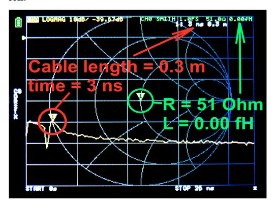
:Finally: a short circuit at the end of teh test cable:
