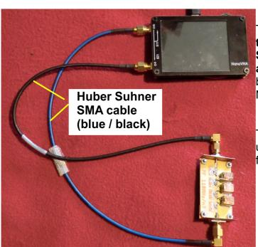
The solution is to purchase and to use two very high quality cables (Huber Suhner with blue black outer), they are specified to 18GHz. They should be permanently attached to the NanoVNA.
