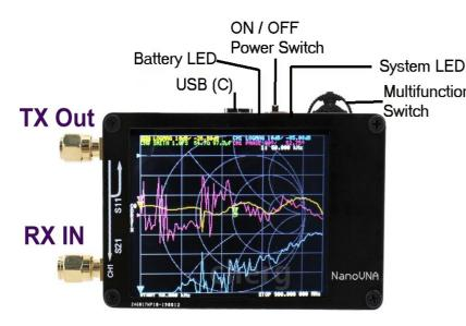
On the left there are two of SMA sockets: the RF input and output. The upper Multifunctional socket is the transmit port Switch (CH0) and is also the channel for S11 measurements (reflection).
