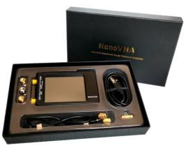
b) The hardware is also modified (e.g. better screening of the inputs). But the most interesting points are an extended frequency range up to 1500 MHz and a higher accuracy. Do not forget: you can also buy a metal case shielded version and a larger display with 4.3 inch diagonal.
