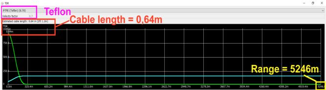
The result of 0.64m =640mm is inaccurate (...result too near toZero). The range rises up to **5246m.**
