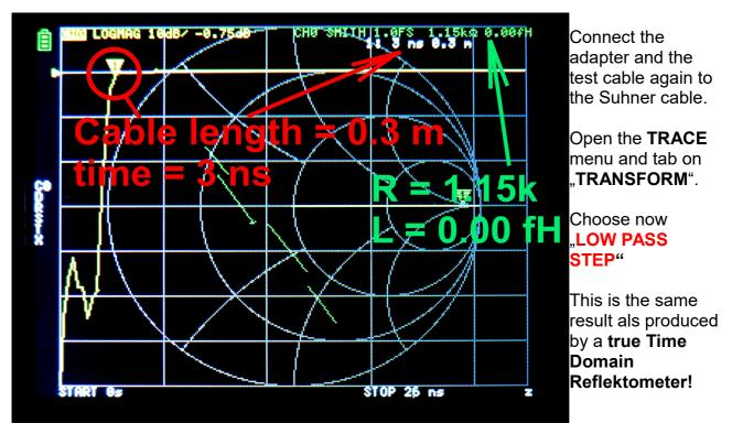
After 3 Nanoseconds (cable length = 30cm) the curve is jumping up to the "Open End Status" with and open end impedance of  $1.15k\Omega$  (= green information at the upper edge of the screen)
