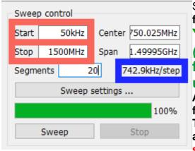
Start with entering the **desired start and stop frequency** in the upper left half of the screen:
