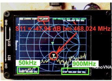
Now press the **Multi Function Switch**(MFS) to the right and hold it there. The marker moves from the start at 50kHz towards the higher frequencies. Try **f** = **468MHz**, it will show 468.042MHz. The display has a scale on the left hand side with 10dB divisions as well as the top "Zero dB point".
