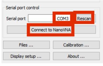
Turn the NanoVNA on and establish the USB connection to the PC by clicking on "Connect to NanoVNA" on the PC screen (bottom left). If necessary with rescan to make sure that the valid USB port is recognised.
