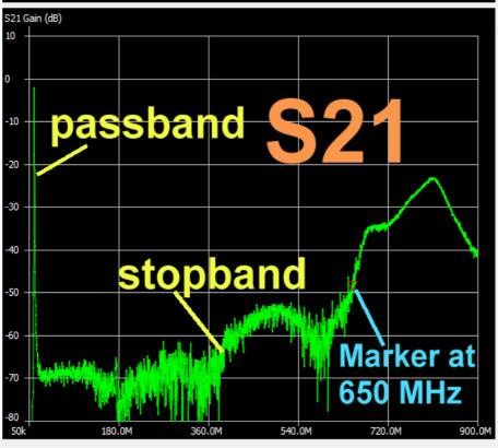
The rest is a problem caused by self resonant effects of the parts.
