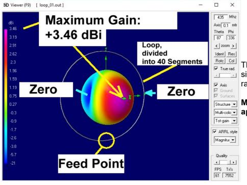
This is a 4NEC2 simulation of the 3D radiation pattern.
