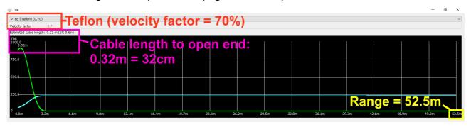
At first the properties of the Teflon cable must be set (red frame).
