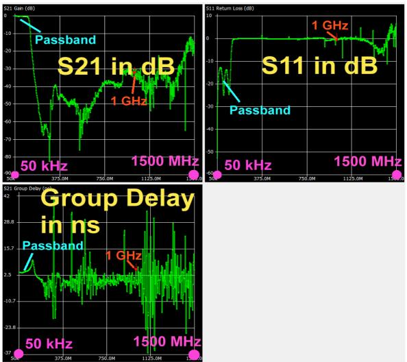
This is **S11** for the **50kHz** to **1500** MHz frequency range. The passband can be identified without any efforts (= low reflection) and in the **stop band** we get a **total** reflection with **S11** = **0** dB
