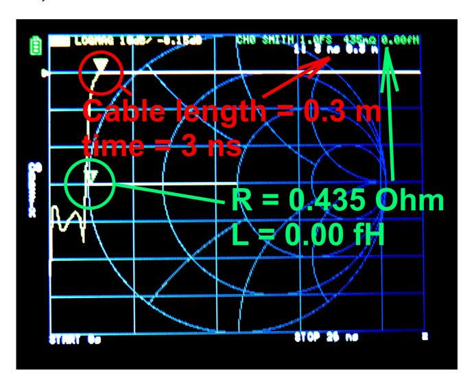
$435m\Omega$  at the cable's end.....this is really a short circuit.....
