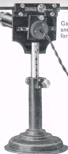
Resistance 10 ohms. Sensitivity 220 mm/ \mu A
