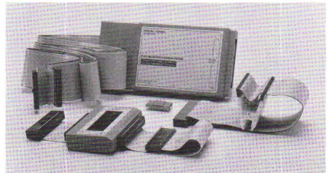
Probe, adapter and interfacing cables for the Z80 microprocessor.
