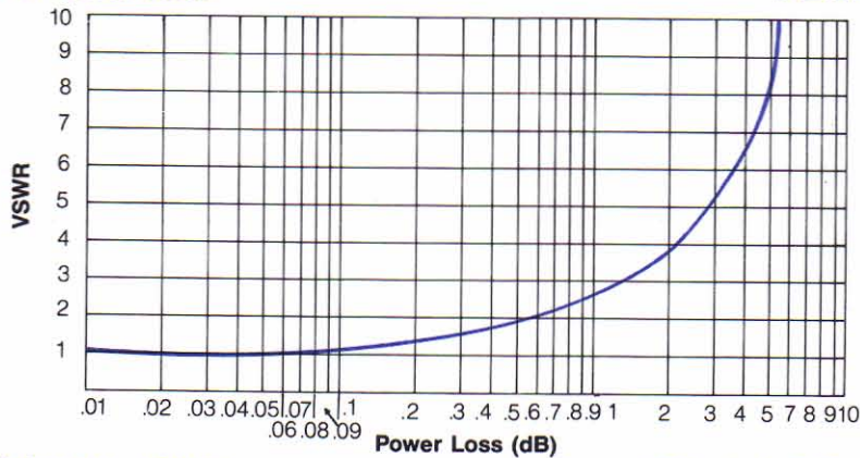
Power Reflected & Power Transmitted vs. VSWR
