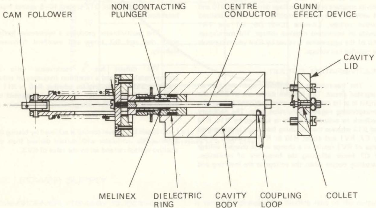
Fig. 8 Cavity Assembly
