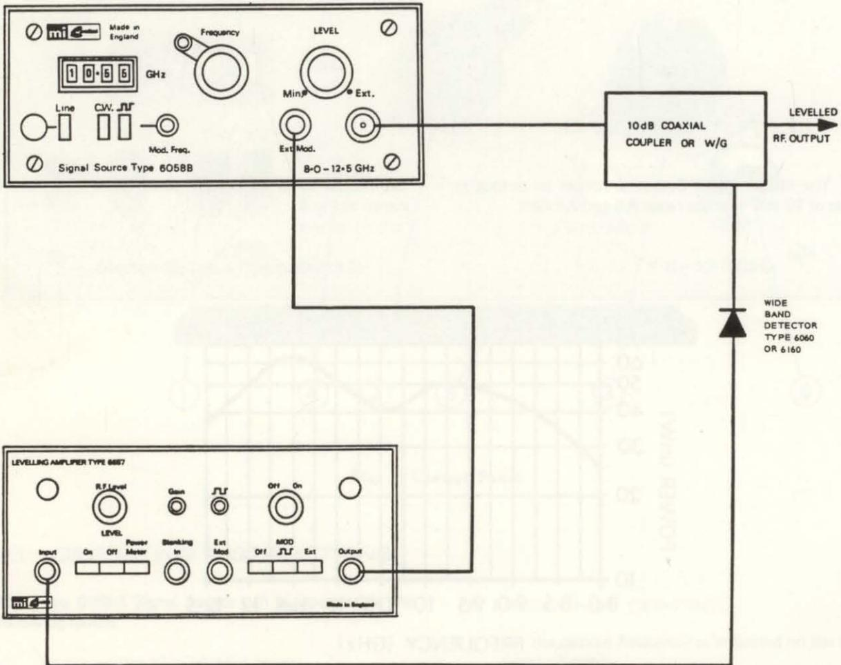
Fig. 4 Levelling Circuit With Type 6587 Levelling Amplifier
