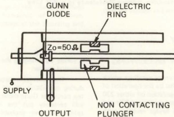
Fig. 6 Microwave Oscillator Schematic
