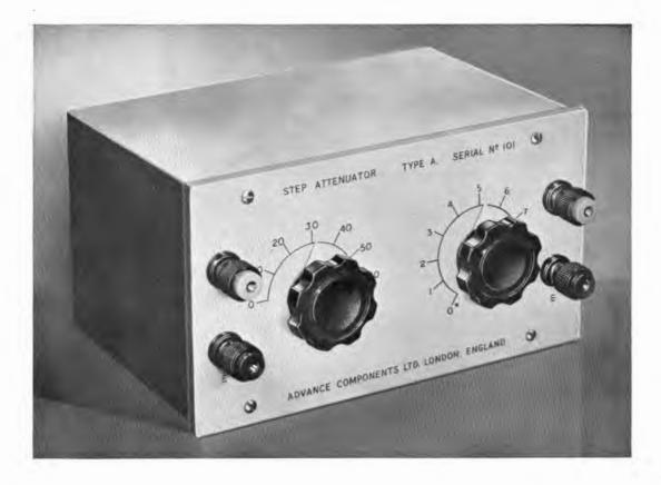
THE type A64 is a variable attenuator with a constant input and output impedance of 600 ohms. It has been designed essentially for use with audio frequency apparatus, but since the errors are still quite small at frequencies at least up to 1 Mc/s, it also has many applications in the telecommunications field. This model is particularly suitable for use with the 'Advance' Audio Signal Generator types J1 and J2.
