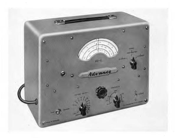
THIS instrument, which has long received world-wide acclamation, completely covers an audio range of between 15 c/s and 50 kc/s with very low distortion. Level output is maintained over its full range.
