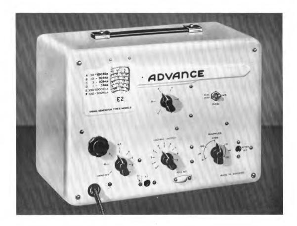
THE most widely used instrument in its sphere, the type E2, which operates entirely on *fundamental* frequencies, is characterised by its exceptionally low R.F. leakage, which even at 100 Mc/s, is less than three microvolts. In addition to internal modulation at 400 c/s, 30%, it may be modulated from an external source to give 0.80% modulation up to 4 kc/s, and 0.40% modulation up to 10 kc/s. The input impedence is 50 k ohms so that little power is required for modulation.
