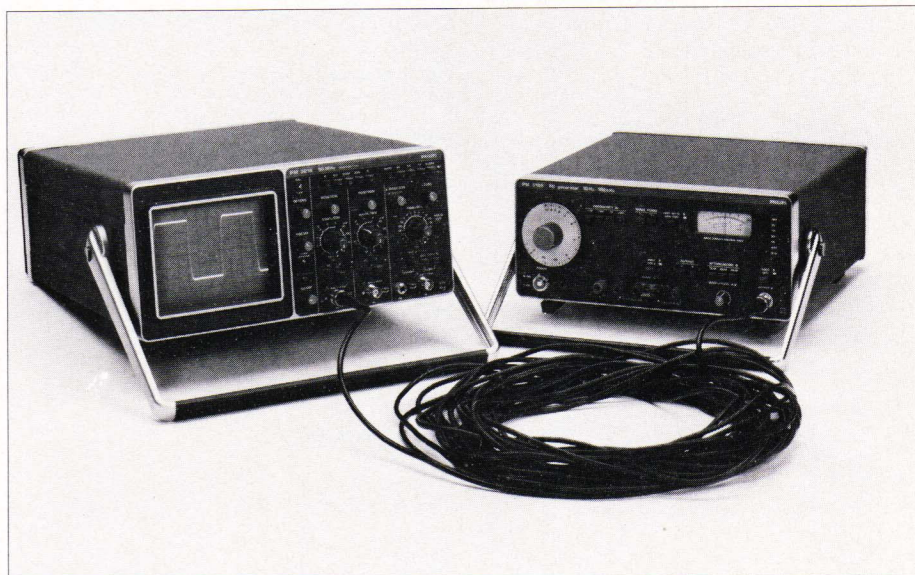
PM 5109 being used to check the bandwidth characteristic of a long coaxial cable.
