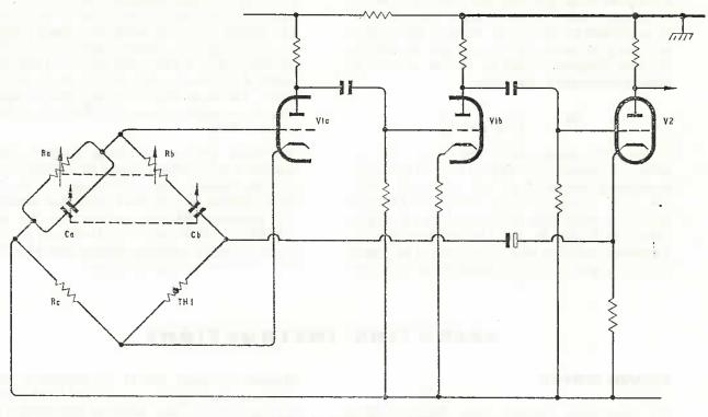
Fig. 1 Basic Wien Bridge Oscillator
