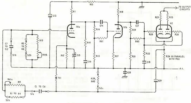
Fig. 4 Oscillator Circuit -- Simplified
