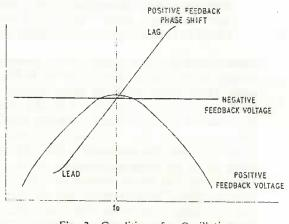
Fig. 2 Conditions for Oscillation
