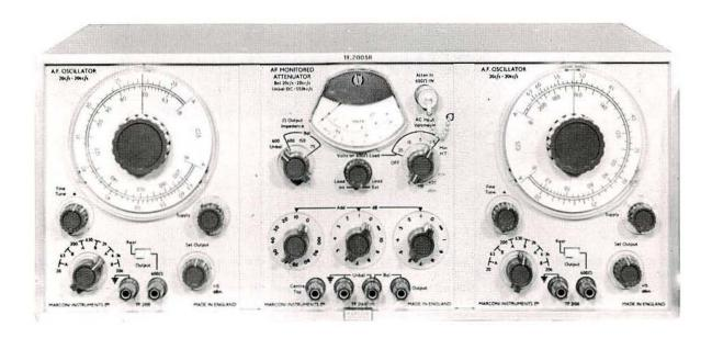
In certain types of a.f. amplifying or transmission equipment intermodulation distortion produced by non-linearity is more important than the harmonic distortion. Standard methods of measurement of inter-modulation distortion have, therefore, been recommended by S.M.P.T.E. and C.C.I.F. The TF 2005 Two-Tone Signal Source is an assembly of standard Marconi modular units arranged to form a convenient test set for measurements following these recommendations.
