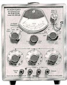
The TF 2160 combines the attenuators with a wide-range a.c. voltmeter and a high quality a.f. transformer so that accurate measurements can be made in the audio band. Without the transformer in circuit the operating range extends up to 550 kHz, and without the voltmeter to d.c.
