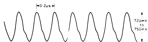
Fig. 4.12 Collector TR1 Schmitt trigger circuit
