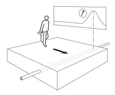
When a signal is detected continue along search route until signal strength reduces, returning to position where signal is strongest.
