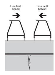
Follow the cable route pushing the A-Frame spikes into the ground at regular intervals and check for a forward pointing arrow.
