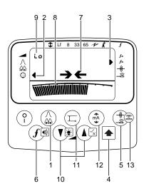
The RD400PXL-2 EMS Receiver is designed to locate buried conductors and 3M markers either simultaneously or independently. Marker location is achieved by the operator fitting an 'EMS Boot' to the Receiver.
