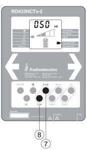
When Multi is selected, any combination of Lf, 8k, 33k and 65k can be transmitted using Direct Connection. The selection procedure is as follows:
