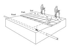
Rotate the A-Frame through 90° and FaultFind along the marked line, until the exact point is found where the arrow changes direction.
