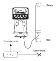
Using the Peak/Null key select Accessory Socket and push the A-Frame spikes into the ground, near the earth stake of the transmitter, with the red spike nearer the ground stake.
