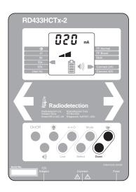
Press the A-V-O key to display current (mA). Press the Up or Down keys to set the required output current level (typically 20 mA). In situations where there is a high degree of interference selecting a higher current may be desirable.
