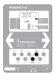
Pressing the Peak/Null key selects either Peak, Null (standard locate modes) or the Accessory Socket when A-Frame is connected.
