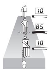
Moving Receiver steadily from side to side, follow line of maximum response, keeping blade vertical and across the target line.
