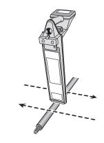
Move Receiver side to side and observe maximum response over centre of signal.
