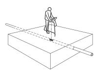
Midway between the spikes mark the ground with a line at 90° to the A-Frame.
