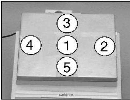
Basic<sup>plus</sup> Balances with laterally installed weighing systems (strain gauge 0,1g resolution) and single-casting block systems (small): The diagram at the left applies to Basic<sup>plus</sup> balances with rectangular weighing pans.
