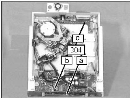
Should there be any defect in the electronics of your Basic<sup>plus</sup> balance, you should not attempt to repair individual components, but rather exchange the entire PCB set (204). The three PCBs together (A,B,C) form a complete unit.
