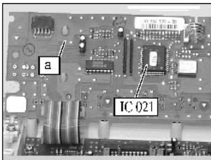
The PCB set (204) is factory-programmed and the PCB-specific data are written onto the AOC (IC 021). Any attempted repair of the PCB would ruin these data.
