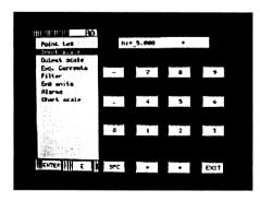
Using the up/down arrow keys select **Output scale** and touch **ENTER**
