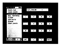
Using the up/down arrow keys select **Eng units** and touch **ENTER**. The alpha-numeric keypad will now be displayed allowing you to enter up to five characters to describe the engineering units for this particular point. For this example
