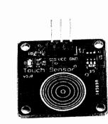
Touch Sensor Switch for Arduino / Pic
