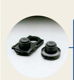
Slide condenser / CX-SLC Brightfield condenser / CH3-CD These Abbe type condensers allow brightfield observations from 4x to 100x. Accurate centering is provided by the attachment lens (CX-AL) and the iris diaphragm, to exclude unnecessary light and obtain bright Koehler illumination right across the magnification range. These highly economical condensers enable phasecontrast and darkfield observations by
