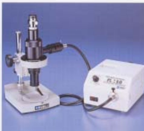
UNIMAC MSL-1FL-PL with FL150 Light Source and FL150/80 Single Arm Light Guide
