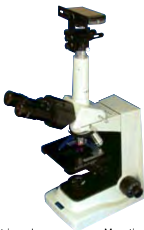
Mounting example of trinocular straight tube stereomicroscope
