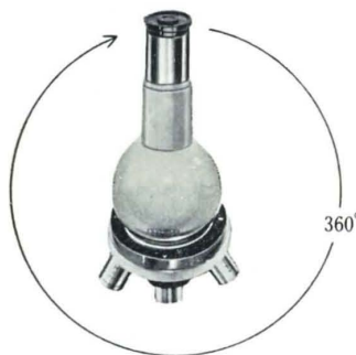
Range of adjustment of direction of microscope head
