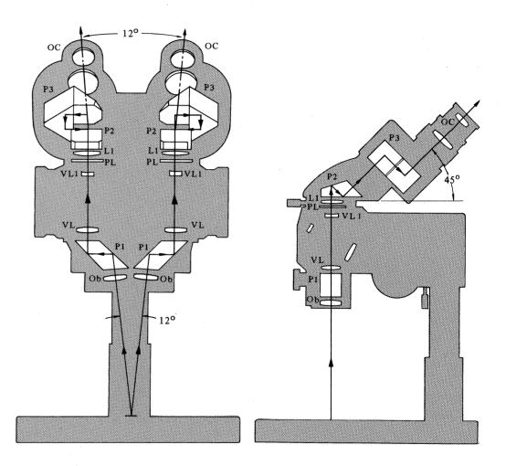
Light bundles from the specimen enter Prism P1 with an angle of visual axis of 12°, where they are turned parallel to each other, then proceed to the variable lens system (VL and VL1), the tube lens system (PL and L1) and to Prism P2. Then, still maintaining parallel position, they enter Porro-prisms at P3, at the last facet of which they again assume a 12° angle of visual axes, forming an image at the eyepiece exit pupil.
