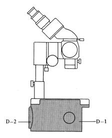
This device provides trans-illumination from below the specimen, when positioned under the stage. It comprises a sub-stage base (D-1), a light source (D-2), and a pair of armrests. An iris diaphragm is also available as a special accessory.
