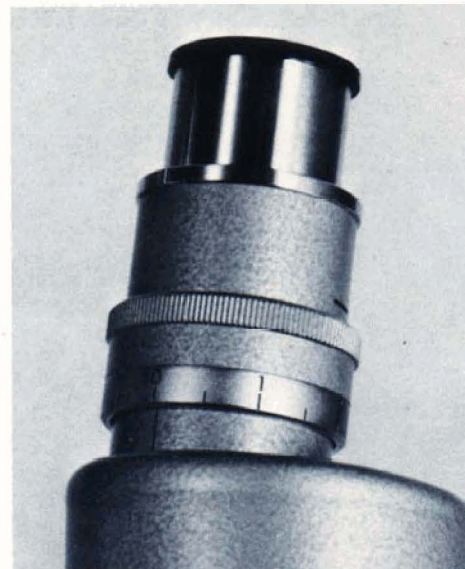
6. Diopter adjustment ranging between +2.5 and -2.5
