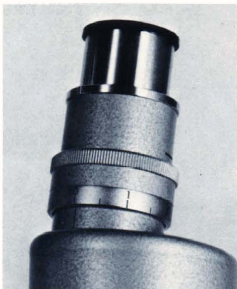
6. Diopter adjustment ranging between +2.5 and -2.5
