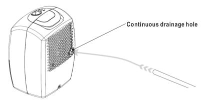
1)Put in the PVC hose into the back of the closed hole, then connect the PVC hose to the front.
