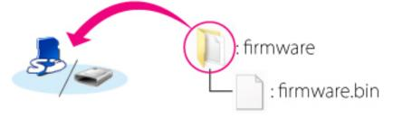
When copying is complete, open the "firmware" folder on the memory card and confirm that it contains the file "firmware.bin".
