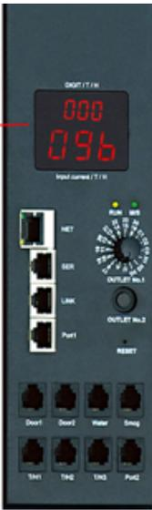
Series number checking method: turn "OUTLET NO.1" knob to "U" on the panel and press the RESET button, then the digital tube will show the series number after the baud rate "9600". The series number is made up of six numbers, letters or number-letter combinations.
