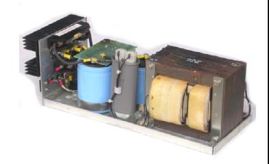
The 2 x 40 Ohm bleed-resistors get hot and may show a mild scorch on the PCB. Adding a fan will help the whole PSU cool under continuous use and/or these resistors can be remote connected to a heatsink etc. These details are application specific and the user's
