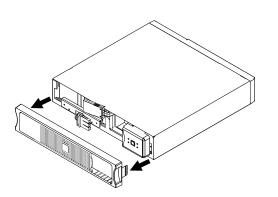
2 Remove battery bracket screws, battery bracket, and battery.
