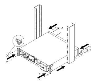
Reinstall battery, battery bracket, and screws.
