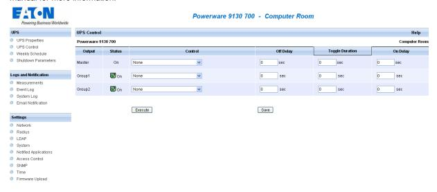
This page enables triggering of startup and shutdown sequences for the UPS main output and controlled outlets.
