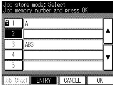
The screen displays 5 job number keys on the left. Arrow keys (▲/▼) on the right side can be used to scroll through the 15 job numbers.
