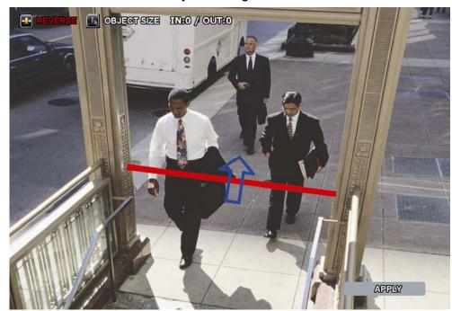
Step2: Click **APPLY** to finish the IVS setting and return to the live view. The IVS icon ""will be shown on the status bar. Click it to show the flow counting on the top left side.
