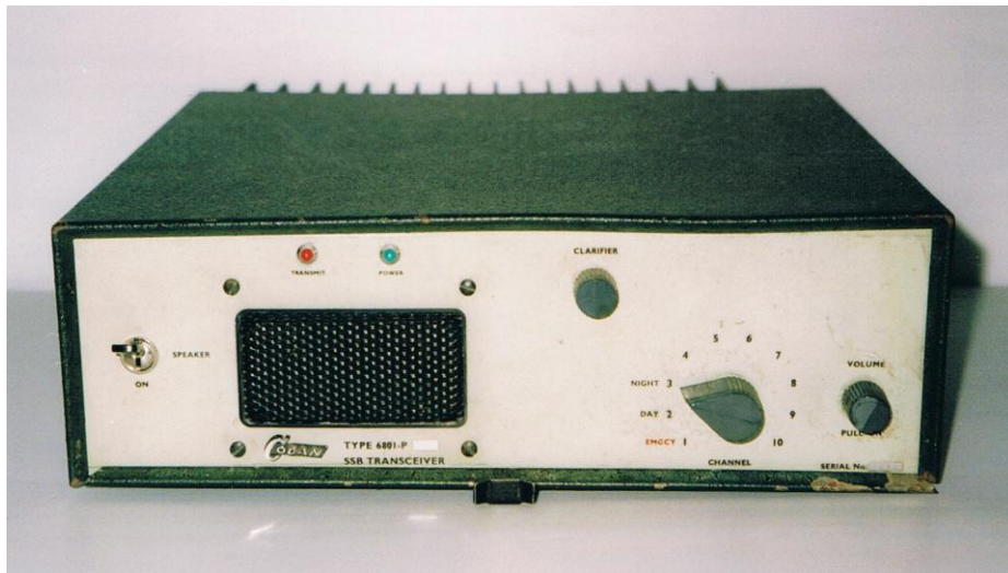
Figure 1 Type 6801 SSB set, 5 channels, 100 watts PEP
