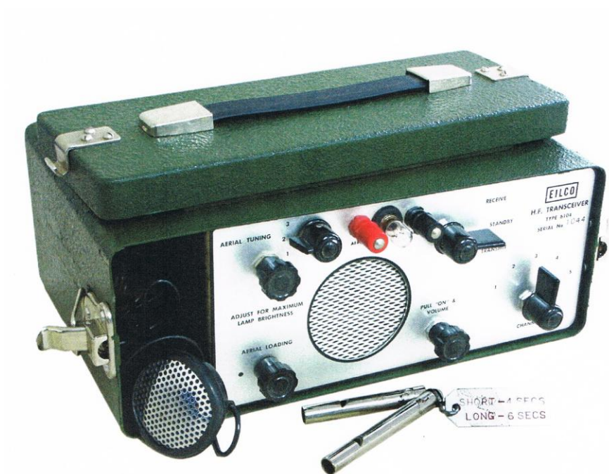
Figure 1 Type 6801 SSB set, 5 channels, 100 watts PEP
