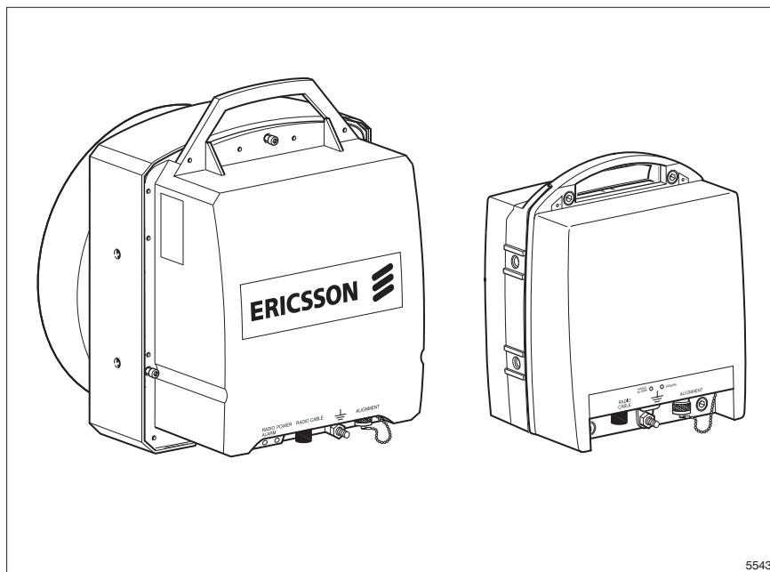
Figure 2-3. RAUs with integrated antenna
