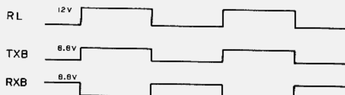
Fig. 10 STANDBY keying timing chart
