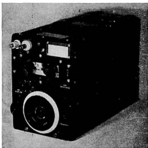
Front view of the heterodyne v.f.o., showing the 2E26 tuning control and the band switch mounted on the plastic window.
