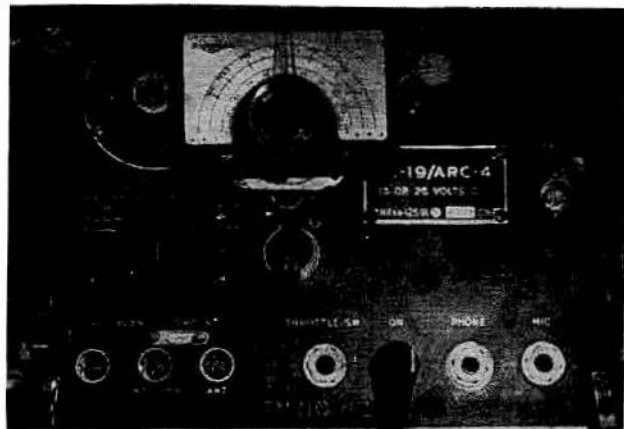
Front Panel of the converted ARC-4. Note position of tuning dial and volume control.
