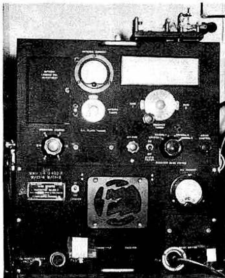
Front view of the BC-669. The upper deck contains the transmitter and receiver and the lower deck houses the modulator and speaker.
