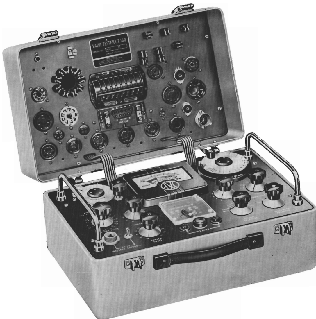
THE AVO VALVE TESTER TYPE 160
